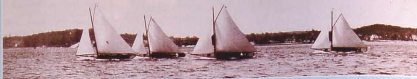
A fleet of New York 30s charges to windward during the class's first season, 1905. The design's bowsprit was lengthened by 2' after this first year, to reduce weather helm.
